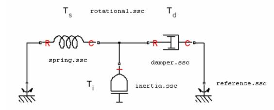
The domain is declared in a file named rotational.ssc (see "Example — Declaring a Mechanical Rotational Domain" on page 2-11). The following file, named spring.ssc, declares a component called spring. The component contains:
