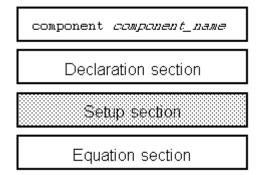
The setup section of a Simscape file follows the declaration section and consists of the function named setup. The setup function is executed once for each component instance during model compilation. It takes no arguments and returns no arguments.
